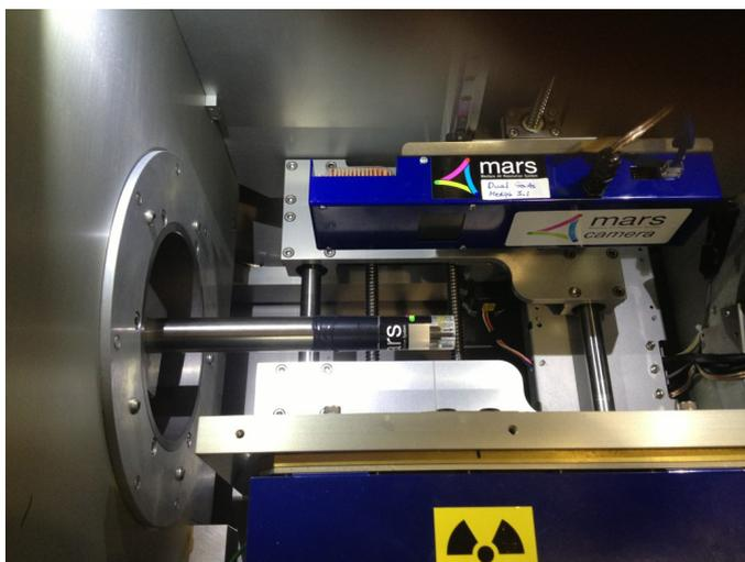
*Fig 2: Gantry of the MARS-CT with the X-ray source and the MARS camera and with a sample placed in between.*
