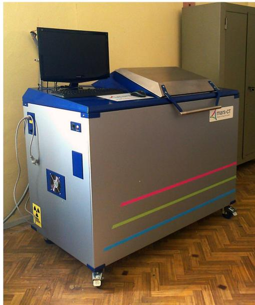
*Fig 1: General view of the MARS microtomograph located at the Laboratory of Nuclear Problems of JINR*
