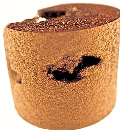
*Fig 3: Image of the rock sample reconstructed at the MARS-CT at JINR (diameter of the sample is about 1 cm.)*
