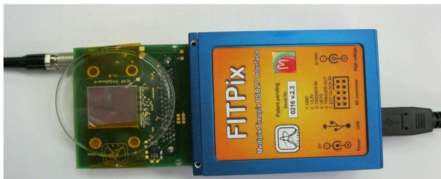
Fig.1 The hybrid pixel detector Timepix with USB interface FITPix
