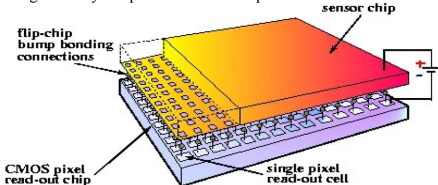
Fig.2. The structure of the Timepix detector
