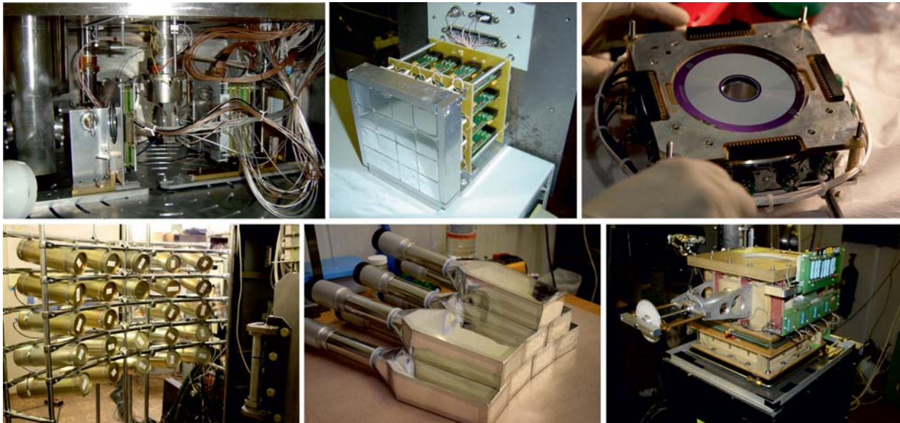
Fig. 2. Some instrumentation available at ACCULINNA: Opened reaction chamber view, charged particle telescopes, stilbene neutron detector array, GADAST \gamma -detector array, and Warsaw OTPC.
