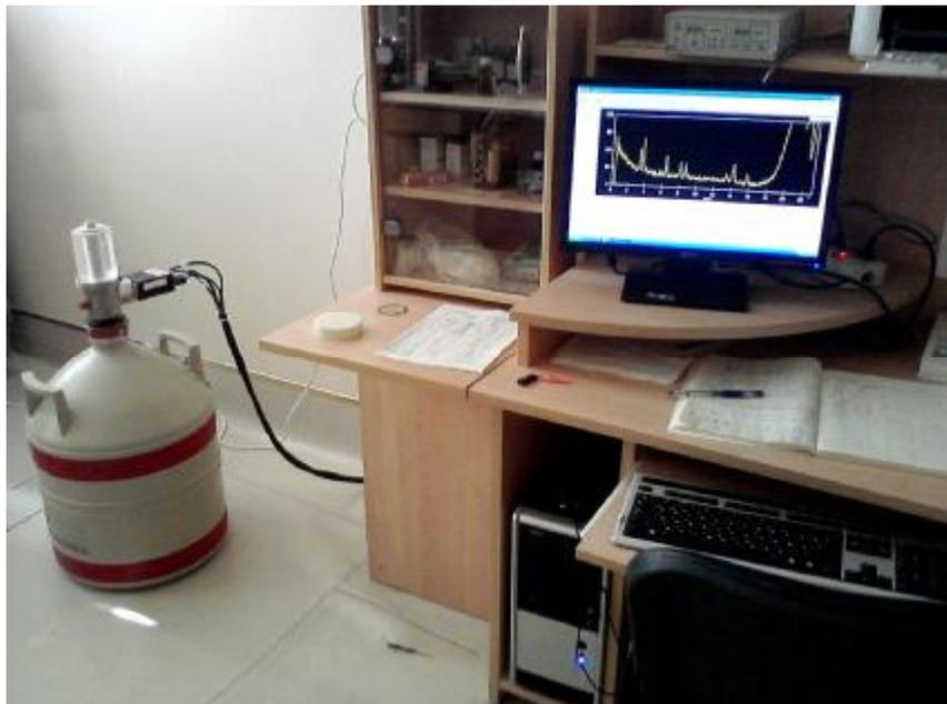
X-Ray Fluorescence analysis of the soil samples will be carried out by the X-ray fluorescent spectrometer at FLNR, JINR
