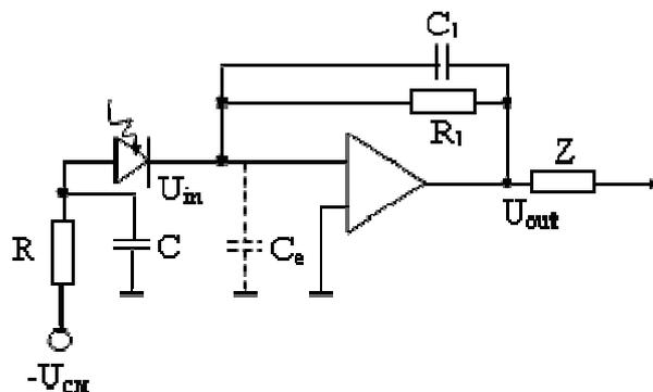
Fig.2. Simplified scheme of charge-sensitive preamplifier.
