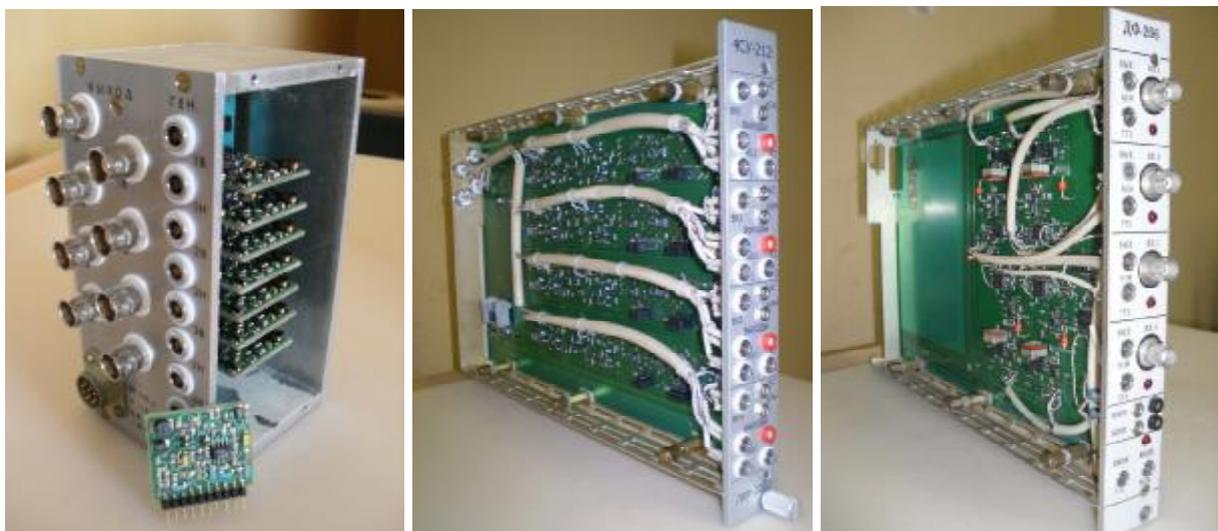
Fig.3. The 8-channel charge-sensitive preamplifier; the 4-channel spectroscopic amplifier; the 4-channel fast amplitude discriminator with common threshold level setting.
