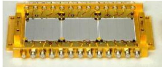
Fig.1. Position-sensitive 12-strip focal plane detector array of the Dubna gas-filled recoil separator.
