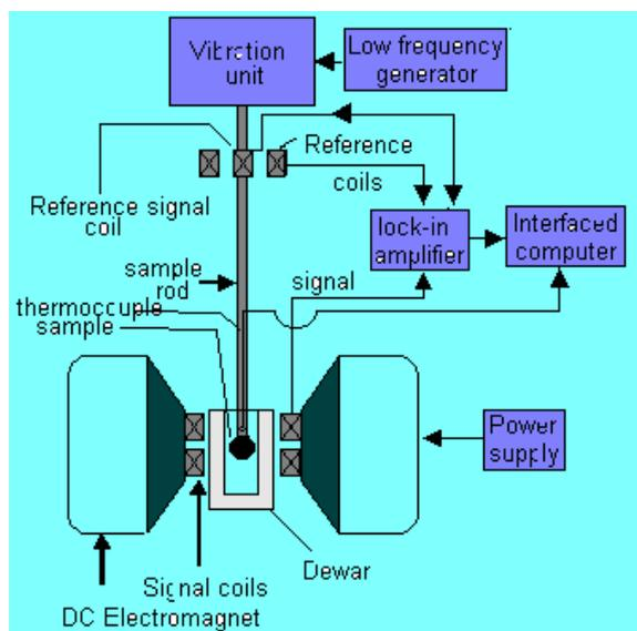
Figure 4 The simplified schema of vibrating sample magnetometer
