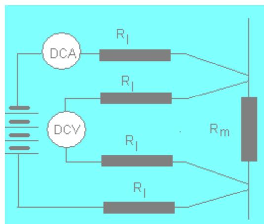
Figure 5 The simplified schema electrical measurements (environment and computer connections are not presented)
