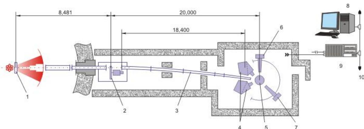
Figure 3. High resolution Fourier diffractometer (HRFD) 1 – Moderator; 2 – Fourier Chopper; 3 – Guide Tube; 4 – Main Detector; 5 – Sample Position; 6 – 90°-Detector; 7 – PSD Detector; 8 – VME Control and Operative Visualization/Analysis; 9 – VME Station (OS/9) Data Acquisition; 10 – Ethernet Data Transfer (Figure from <http://flnp.jinr.ru/136/> site)
