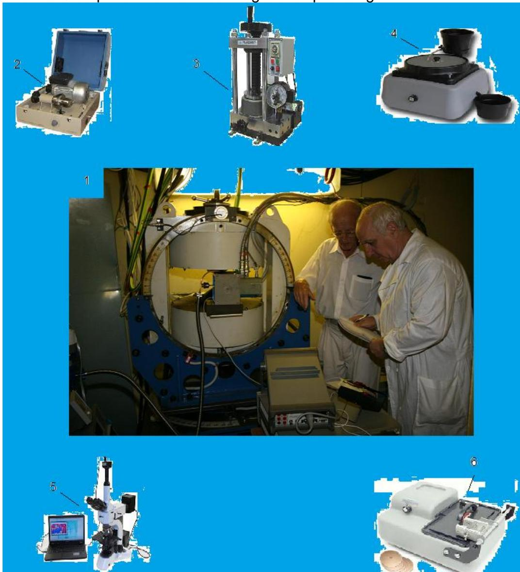
Figure 2 Some instruments used to obtaining manganites and determining their transport properties. 1. General view of installation for magnetoresistance measurements (photo 2008, on YUMO electromagnet; today (2012) installation is near HRFD); 2. High Speed Vibrating Ball Mill; 3. Electric Hydraulic Laboratory Press; 4. EQ-Unipol-300 Economic 3" Grinder / Polishing; 5. Metallurgical microscope; 6) High Speed Diamond Cut-off Saw
