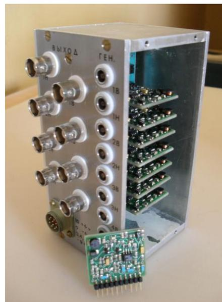
Fig.3. Preamplifiers' box for a position sensitive detector
