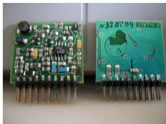
Fig.4. Charge-sensitive preamplifier for the one channel of the detector
