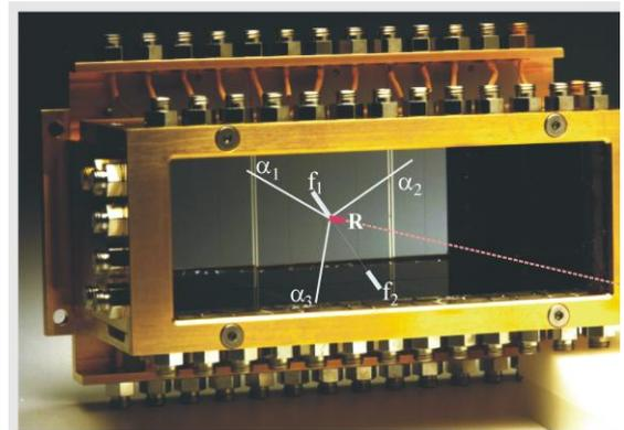
Fig.1. Focal plane detectors array
