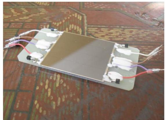
Fig.2. Si position sensitive PIPS detector
