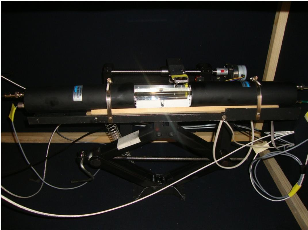
Fig.1. The single crystal scintillation detector
